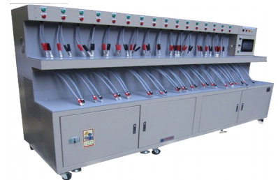
NTCDR-150-80-150-10CH DICHARGE TEST MACHINE
