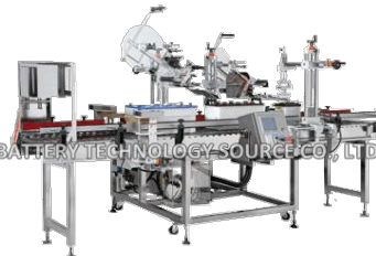
BL-20AC FULLY AUTO. CAR BATTERY LABELING MACHINE
