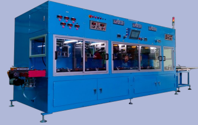
HV-60AM (X) FULLY AUTO. POLARITY CHECK, INTER-CELL WELD, S/C & WELD QUALITY CHECK MACHINE (WITH SERVO CONTROL)
